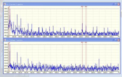
When signals appear in the 500 to 2000 Hz range the bearing is now a late stage 2 defect.
